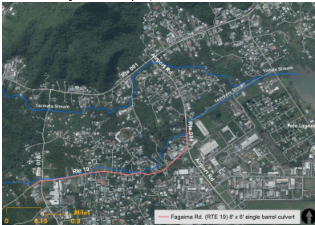
Figure 8: RTE 19/Fagaima Road flood mitigation project
